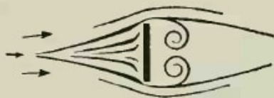
Water flowing round an obstructing plate or slab (after Isaachsen)
