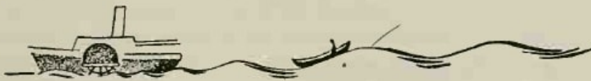
The boats of the natives perch on the waves in the wake of a steamer and are carried along by them (after Idrac)
