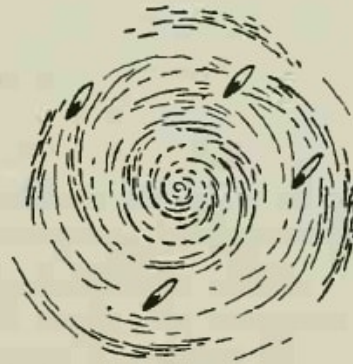
A small piece of wood circling in a vortex. It constantly points in the same direction
