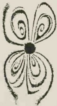
An object moved backwards and forwards in water creates a field of vortices
