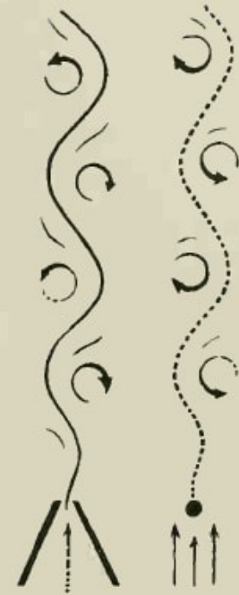
Comparison of two vortex trains from different causes: the direction in which vortices spin varies according to whether they are caused by an obstacle obstructing a stream of water or by a narrow stream of water entering still water through a small opening. The pattern of the vortices remains the same
