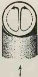
Secondary currents in the bend of a pipe or of a wide blood vessel
